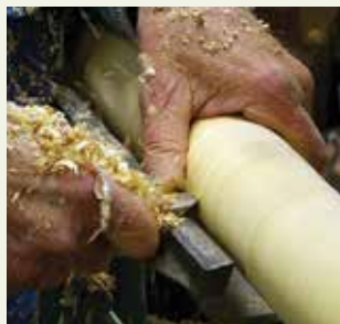
(Bottom) A round-nose scraper is Myron’s tool of choice. He has spent more than eighty years at the lathe, most recently as a production turner.
